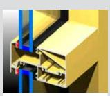
Full captive wedge glazing is a feature of 426 framing. We can use silicone wet top on the outside in lieu of the captive wedge.
