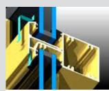
Concealed drainage designed to shed water more efficiently and improve aesthetics without runs of visible holes along the face. Very high water performance > 600 Pa.
