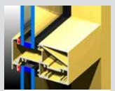
Full captive wedge glazing is a feature of 426 framing. We can use silicone wet top on the outside in lieu of the captive wedge.
